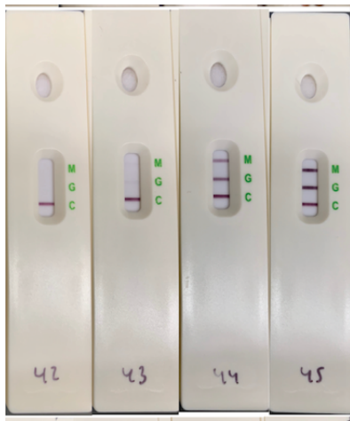
Figure 5: Representative photo of SARS-CoV-2 LFA results. Note, Sample 42= Negative (0), Sample 43= Weak Positive (1), Sample 44= Positive (2), Sample 45= Strong Positive (3)
